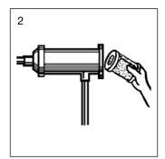
$\triangle$  The standard gasket of the CCY (neoprene) is not compatible with CO<sub>2</sub>. Use the reference CY 15555200.
